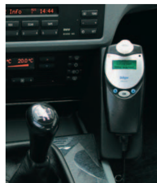
Dräger Interlock XT: Fits in the dashboard.
